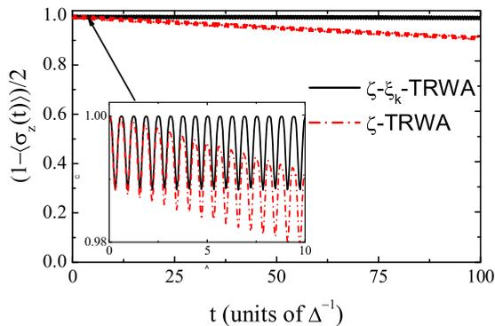
FIG. 10. (Color online) The probability of the TLS remains in its initial state as a function of  $t$  is shown for  $\alpha = 0.01$ ,  $\omega_L = 10\Delta$ , and  $A = 24.0483\Delta$ .
